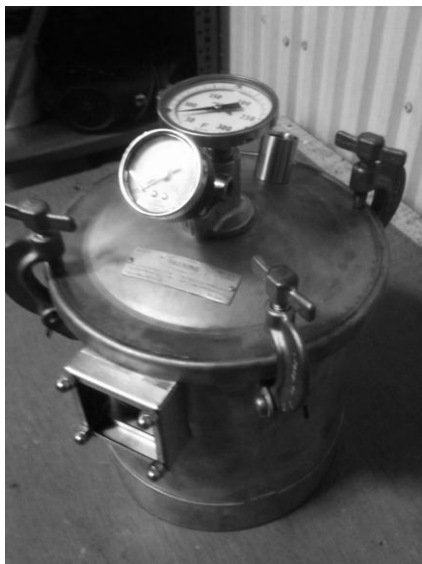
The gasification apparatus itself
