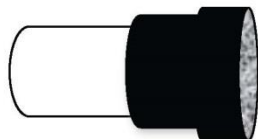
Figure A: The black coupling attaches to the pipe to secure the filter and withstand pressure. The larger end of the coupling contains the material components of the filter.
