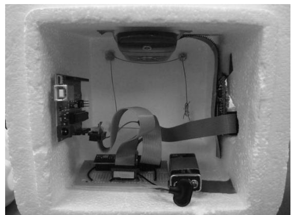
Figure 2. In the figure above the final configuration of the components is shown. Immediately before launch a heat source would be added to maintain core temperatures. The CO 2 sensor is mounted on the right wall inside the hole. The remaining features were
