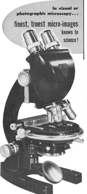
You get clear, sharp, distortion-free images with the superb apochromatic objectives of Bausch & Lomb Research Microscopes, Entire optical system is BALCOTED to eliminate internal reflection and minimize flare . . . to ensure image brilliance. Slow-motion, lowposition fine focusing adjustment assures lifetime mechanical accuracy. Choose from the complete line, for general or highly specialized studies.
