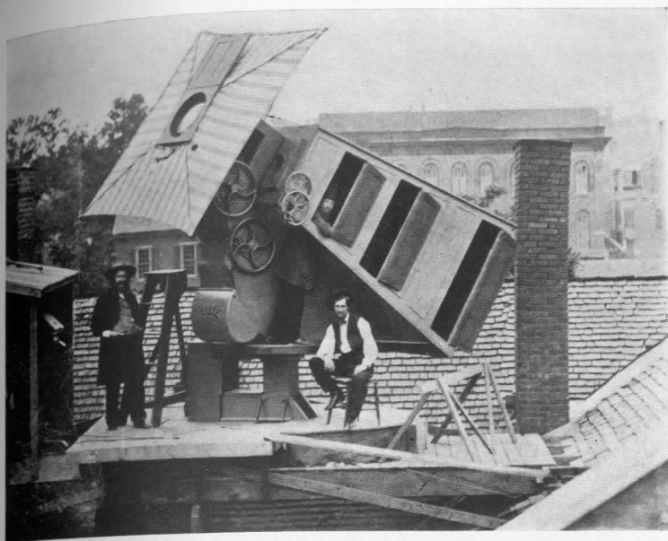
Barnard's first photographic work, about 1866, was to keep this enlarging camera pointed toward the sun. The man at the left is Van Stavoren, the proprietor, and the man in the camera is J. W. Braid.
