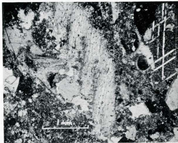
Plate I: A. Photomicrograph of Laminated argillaceous limestone from Locality 1 showing microcrystalline ooze and some opaque material. B. Photomicrograph of Dalmanella coquina containing a Dalmanella shell in the center with the "Manila rope" texture. Also present are microcrystalline ooze, sparry calcite some of which shows polysynthetic twinning (in the upper right-hand corner), dolomite rhombs, and an opaque phosphatic gastropod of the genus Cyclora (upper right-hand corner).
